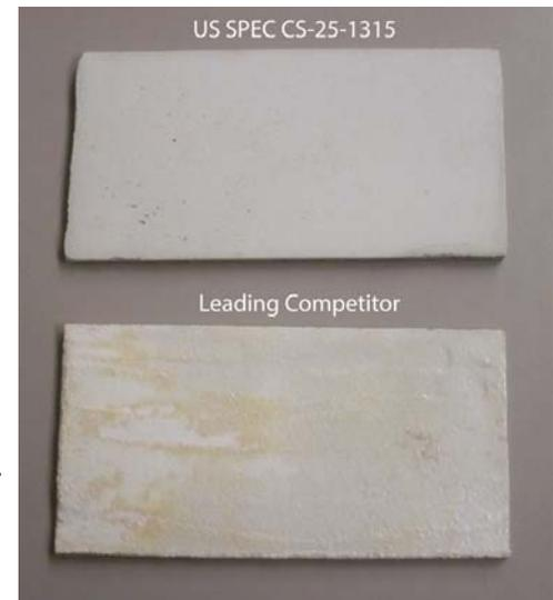
*Panels tested per ASTM C154 via ASTM C1315.*
